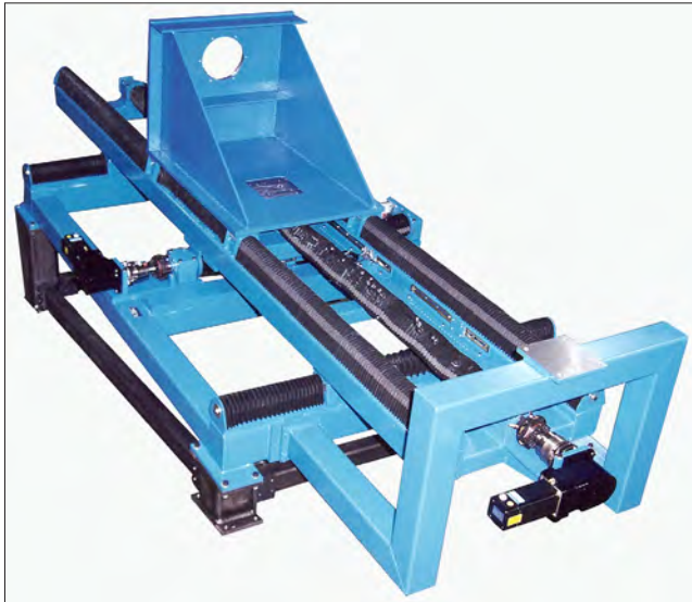
X-Y machine assembly process mounted to steel support structure
